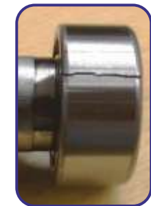
Forced fracture of Outer ring caused by a direct impact blow
