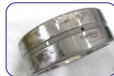
Moisture corrosion on outer ring of Spherical Roller Bearing
