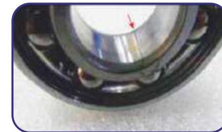
Forced fracture due to excessive interference fit
