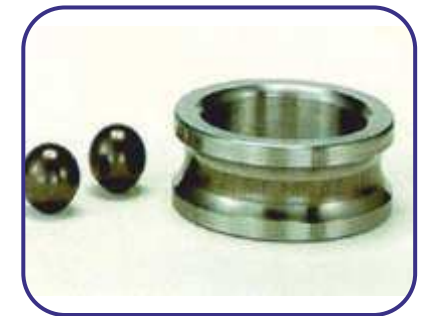
Fluting on inner ring raceway with dark colored balls
