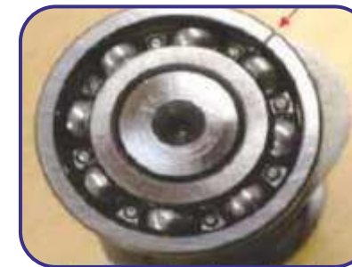
Forced fracture of Outer ring caused by a direct impact blow
