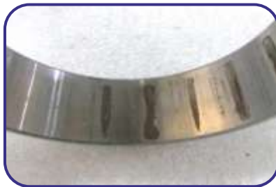
False brinelling and contact corrosion marks on cup raceway of Taper Roller Bearing due to water/moisture entry and vibrations
