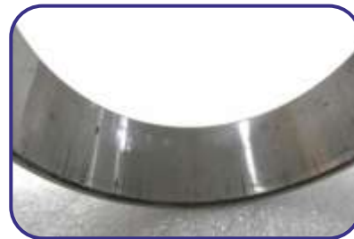
False brinelling marks along with roller dents near large face of Taper Roller Bearing due to vibrations
