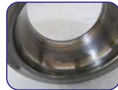
Fretting corrosion on cone bore of Taper Roller Bearing due to micro movement between cone and shaft
