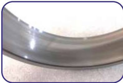
Wear and indentation on cup raceway soft foreign particle contamination
